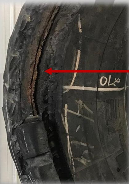
Separation in tire (after being cut out)
